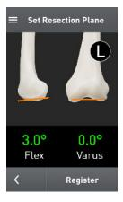
Set desired varus/valgus and flexion/extension angles by using Ball Driver to adjust Microblock navigation screws
