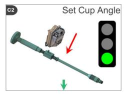
Attach sensor to impactor
